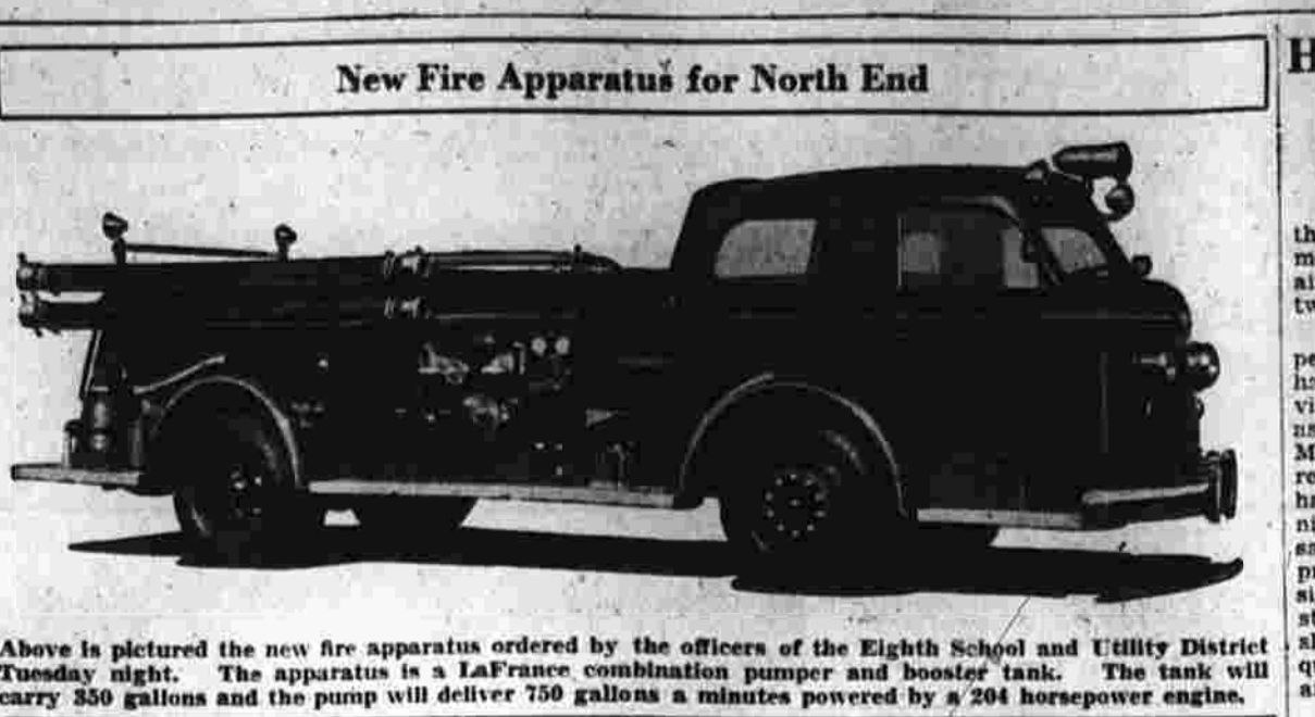
Above is pictured the new fire apparatus ordered by the officers of the Eighth School and Utility District Tuesday night. The apparatus is a LaFrance combination pumper and booster tank. The tank will carry 350 gallons and the pump will deliver 750 gallons a minute powered by a 204 horsepower engine.
